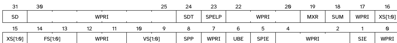
Figure 49. Supervisor-mode status (sstatus) register when SXLEN=32.
